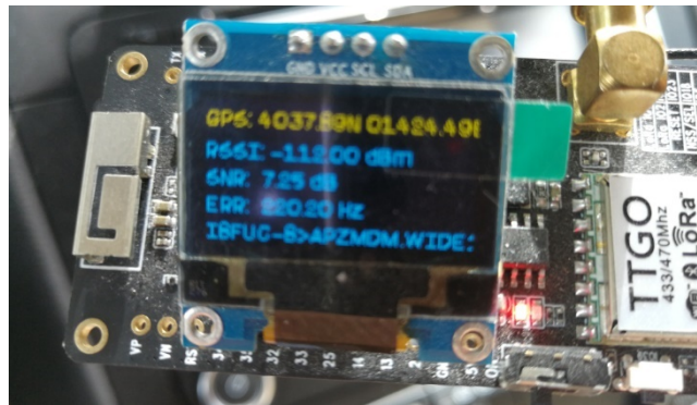
Figure 90 : Example of display content for TTGO T-Beam
