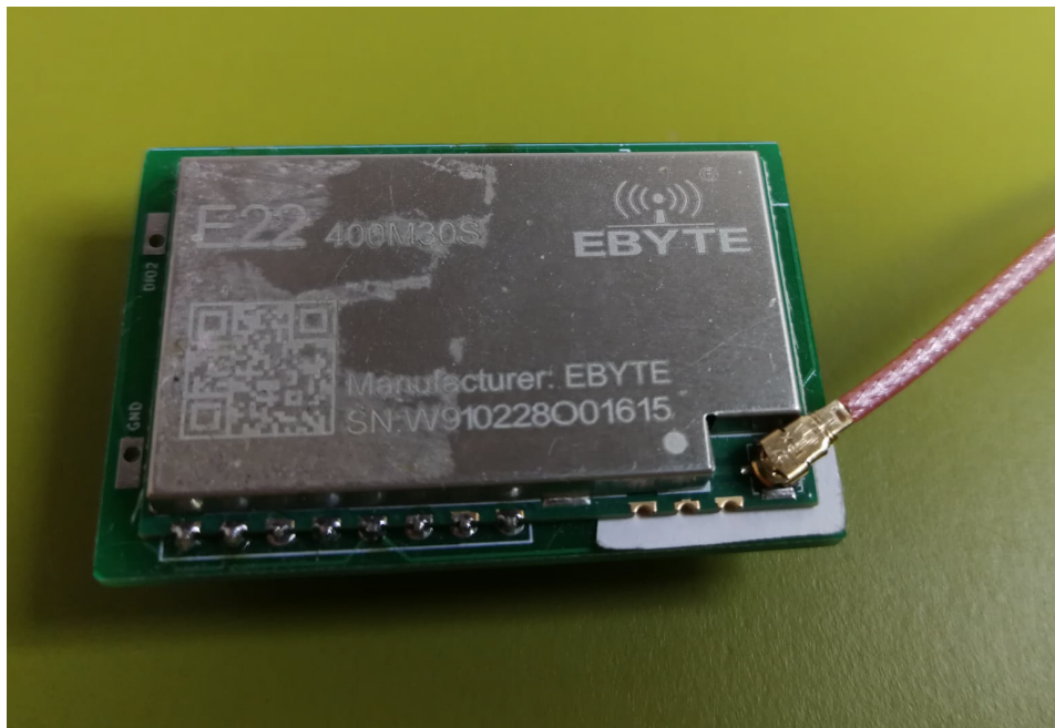
Figure 21: LoRa module mounted on LoRa carrier PCB – view2
