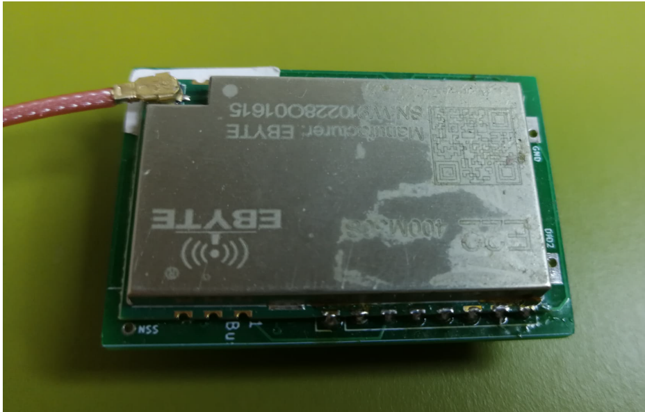
Figure 20: LoRa module mounted on LoRa carrier PCB – view1
